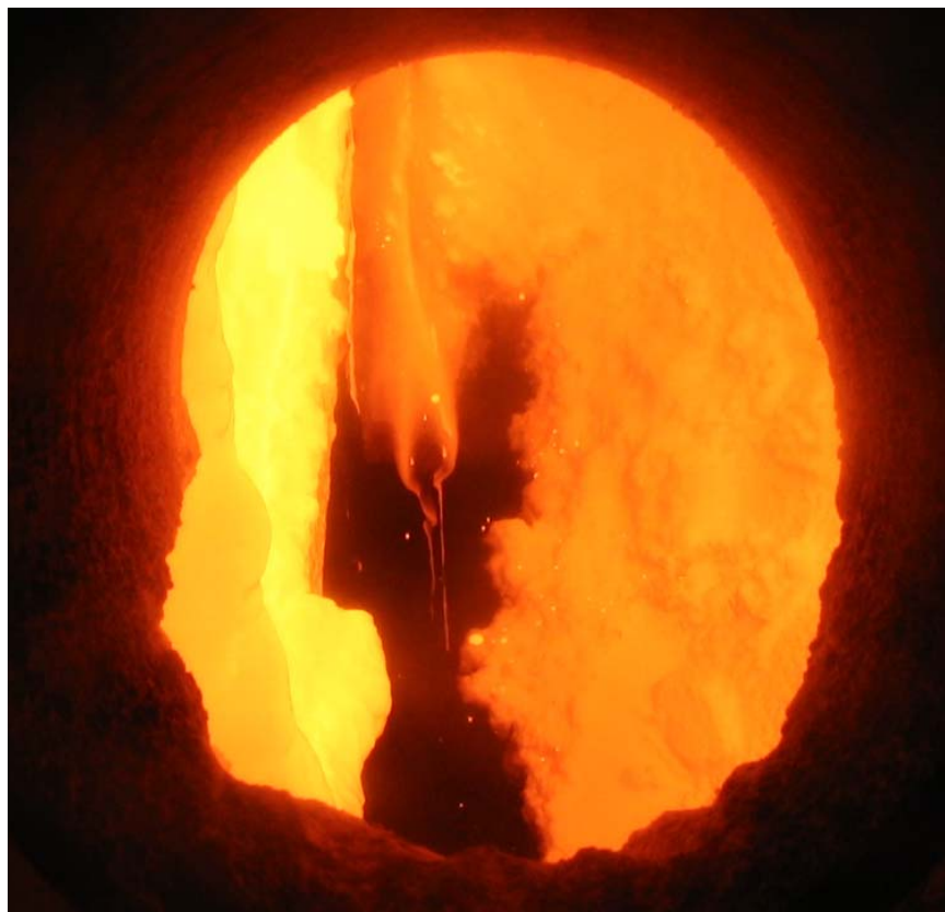
Figure 8. View from Above Drop-Out Box – Molten Slag Dripping from South Wall into the Granulator (kiln nose left, west wall right)
