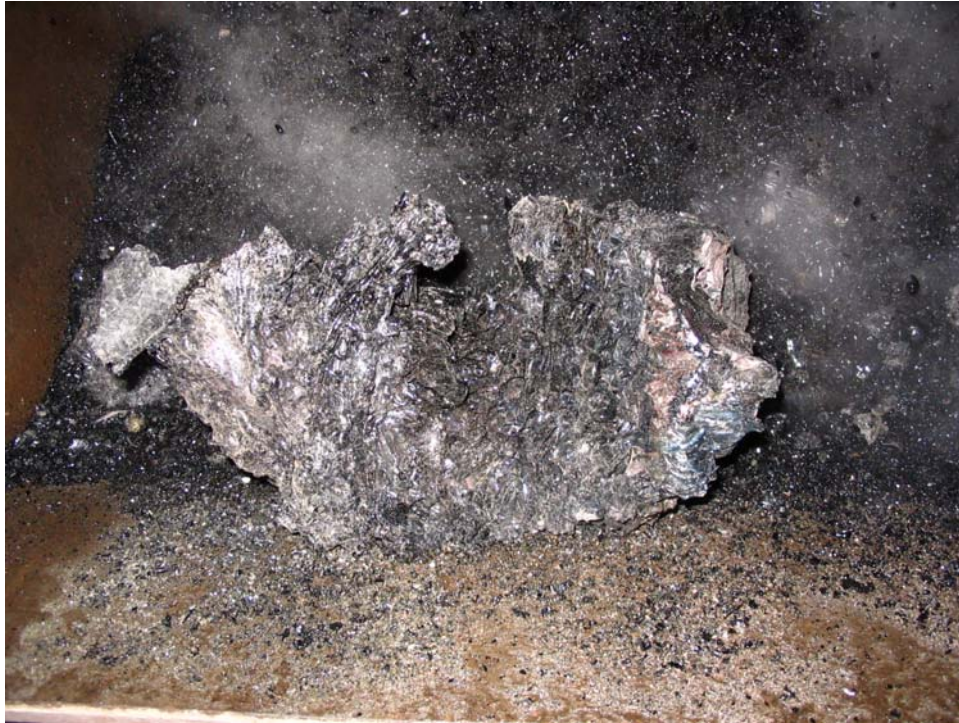
Figure 7. Slag Chunk Cleared from Granulator and Discharged (December 6)
