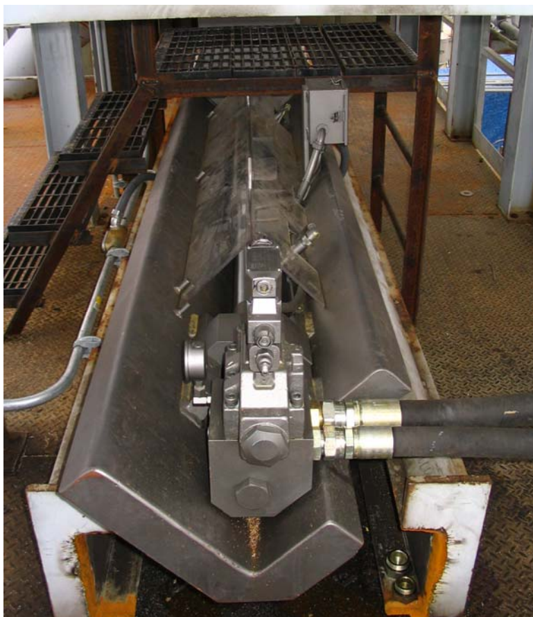
Figure 5. End-View of V-Ram and Hydraulic Connections
