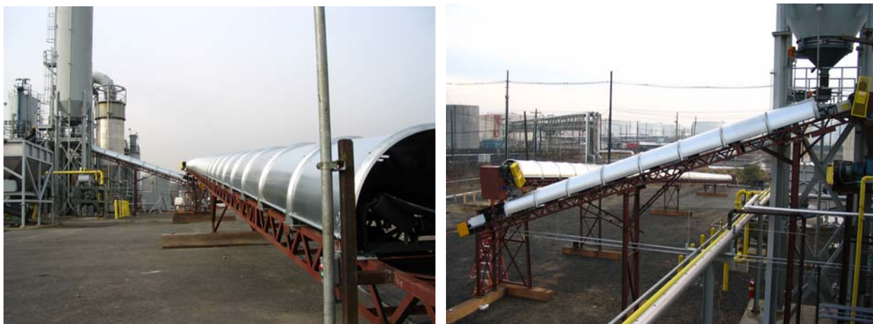
Figure 4. Covered Belt Conveyors Running from the Sediment Storage Area to the Charging Deck (left: looking west from the sediment storage area; right: looking east from the SCC platform)
